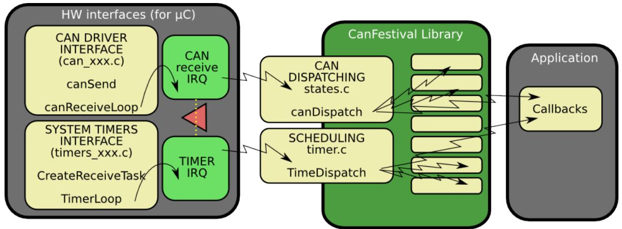
2. OS must provide a receive thread, a timer thread and a mutex. CAN reception is a bloking operation
