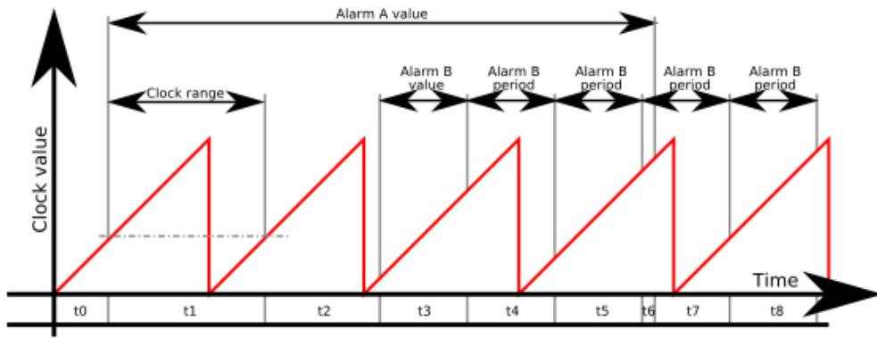
Scheduler can handle short clock value ranges limitation found on some µC. As an example, value range for a 16bit clock counter with 4µs tick is crossed within 0.26 seconds... Long alarms must be segmented.
